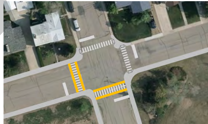
Figure 86. Proper crosswalk striping with stop lines. Yellow lines indicate a raised crosswalk.
