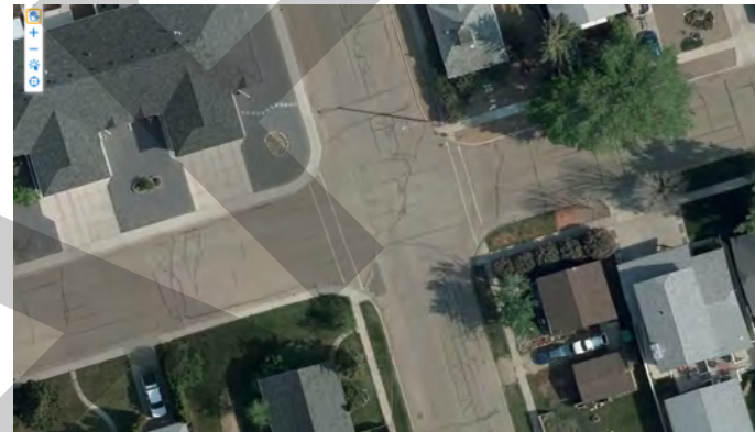
Figure 85. Incomplete crosswalk painting at the intersection of 6 Avenue W and 3 Street W.
