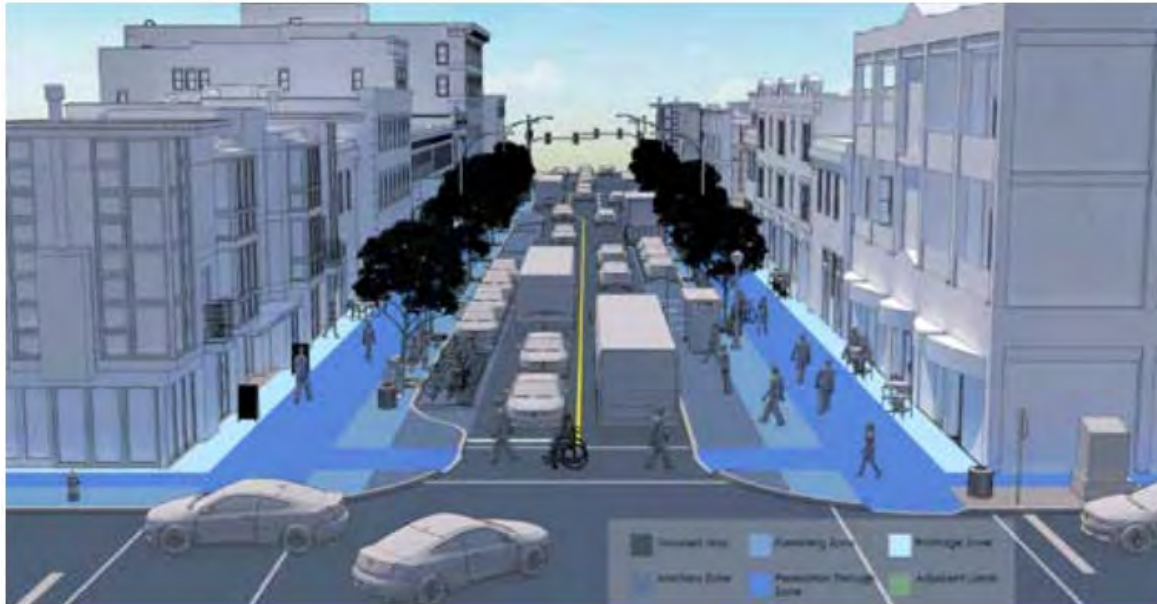
Figure 3 This picture shows the zones for a street oriented commercial road (or a Main Street).
