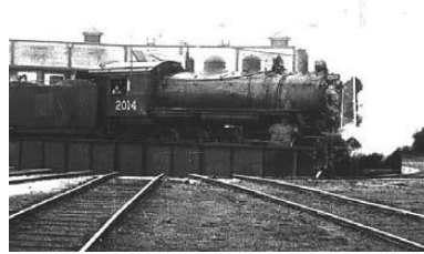
This turntable was used to rotate trains back onto the tracks after servicing
